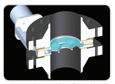
A worm gear rotates the upper ported plate to align its ports relative to ports in the fixed lower plate to increase or decrease the DVO Beta ratio.
