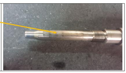
As stated previously, any scoring on the shaft areas that travels between the Seal Cartridge and Actuator Cover will cause o-ring failure, which would cause compressed gas and/or Actuator control medium leaks. O-ring failure that causes compressed gas or Actuation control medium leaks can cause major issues if damaged part replacement and new seal installation is ignored.
