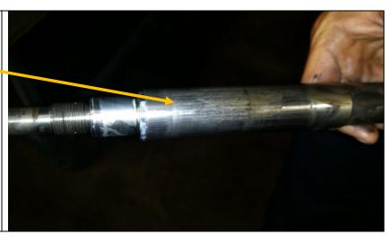
2. Inspect the area of the Unloader Shaft that travels through the Actuator Cover.
