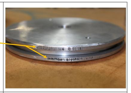
This is an example scoring marks on the inside diameter of the Actuator Cylinder wall.
