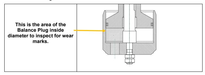
Secondly, check the condition of the Balance Plug where it seats to seal the pocket volume. Damage can occur due to applying a higher than recommended amount of actuation pressure. It is best to refer to the supplied ACI Services assembly drawing for the recommended actuation pressure to apply according to the operating discharge pressure of the compressor.
