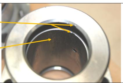
2. Make sure there are no indentions on the outside diameter of the Seal Cartridge. Just like the inside diameter, look for any indentions near the o-ring grooves that could possibly cause o-ring failure. O-ring failure would allow compressed gas to enter the Actuation chamber.
