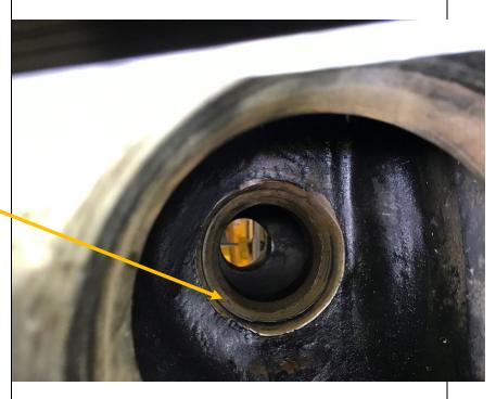
This is an example of a Cylinder Body Pocket seat without wear issues. This seat in particular did not require any repair other than polishing the chamfer.
