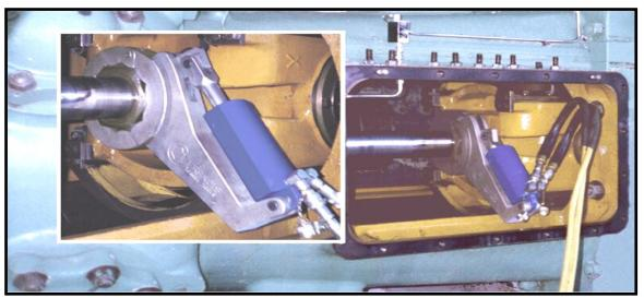
Eliminate hammer wrenching, hydraulic jacks, cranes and other unsafe and inaccurate equipment used for tightening large threaded nuts in hard to
