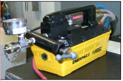
psi air source into as much as 10,000 psi of hydraulic pressure. Exact torque can be preset in minutes and accurately and consistently repeated. A button pendant provides easy advance/extend and retract/return.
