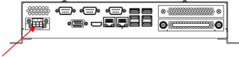
**24VDC Source Voltage Connector**
