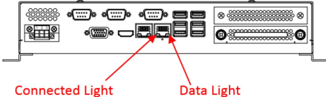
If this is not the case then either data is not being sent or the port is not receiving data. Do the following:
